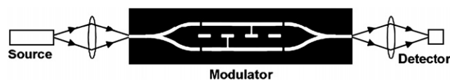
Fig. 2. A schematic of the polymer Mach–Zehnder modulator (top view) with free-space end-fire light coupling. The straight segments in the center (15-mm long, white lines) are the upper electrodes with connection pads; electrodes were not used in the Y-splitter and Y-coupler sections (also in shown in white).
